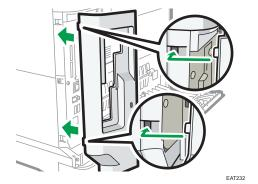
7. Hook the tab on the interface cover, which is located on the side of the rear cover.
