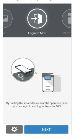
If the login screen is not displayed, press [Settings] ► [Navigation Display Item], and then enable the display of [Login to MFP] on RICOH Smart Device Connector.
