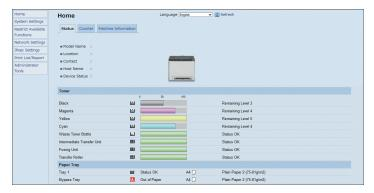
You can check the machine's status and configure its settings by accessing the machine directly using Web Image Monitor.
